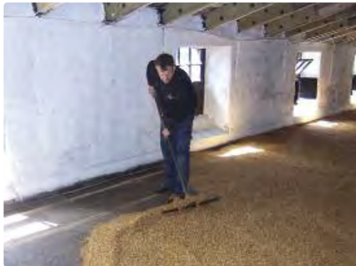
Tartan malt being spread out on one of Highland Park's malting floors in June 2011.
