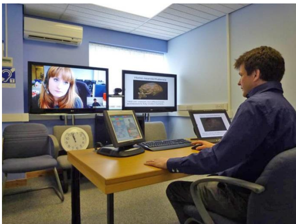
Figure 2: VC with twin monitors and a fixed console being used by the author to make a presentation from Shetland College.
